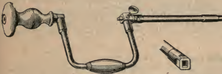
FIG. 44.—BRACE AND BOX-SPANNER.
